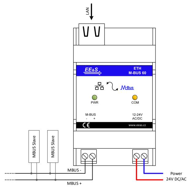
The device is equipped with two LEDs. The green LED labeled as "PWR" indicates the presence of the power supply with a steady light. The yellow LED labeled as "COM" flashes when a packet is sent to or received from the MBUS line.
